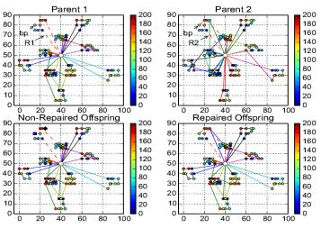
Fig. 2. Sequence-Based Crossover operator with repairing phase (bp=breakpoint).
