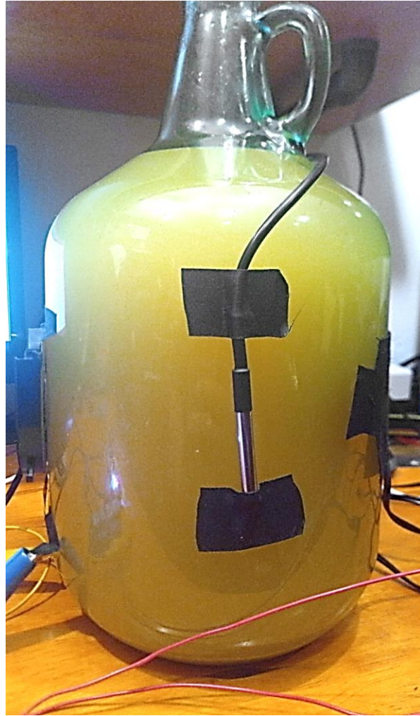
Figure 7 - Temperature sensor attached to the fermenter. Although the most appropriate way to measure the temperature is by inserting the sensor into the beer.
