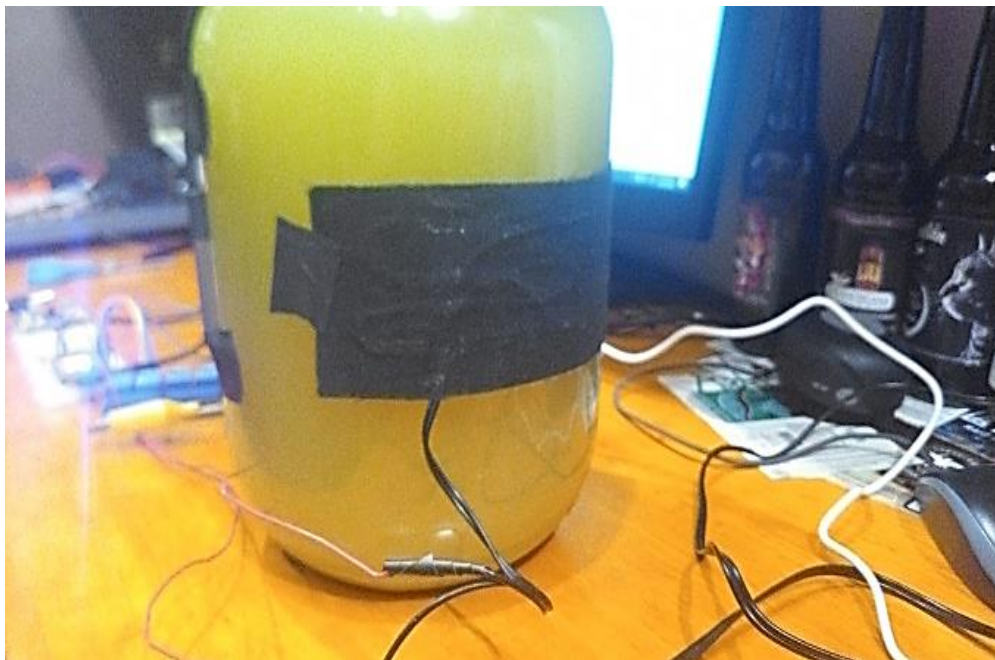
Figure 6 - Heating system consisting of a modified mesh, which is connected to a USB power supply and one of the relays.
