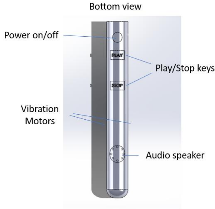
Figure 6. handgrip human interface details
