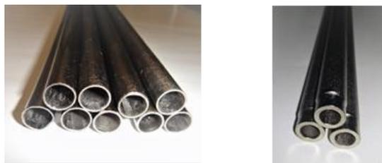
Fig. 4. Copper and 1018 steel tube with coating
