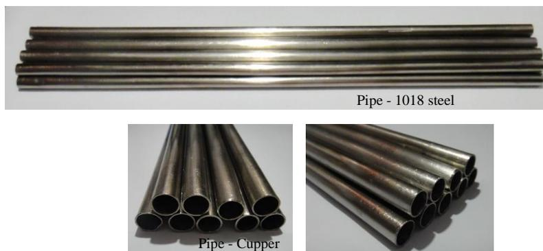
Fig. 6. Copper and 1018 steel pipe with Ni-P coating
