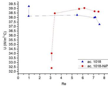
**Graph 4.** Behavior of 1018 pipe steel under normal conditions and with the Ni-P coating
