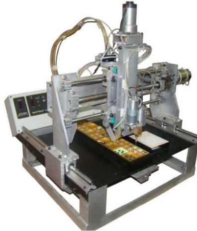
Figure 1. Implementation of a x,y,z Cartesian robot in the modified work area of a MPP-21 manual workstation.
