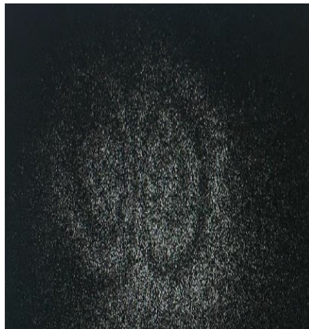
Figure 15. The fringe pattern generated in the region where an internal crack was produced.
