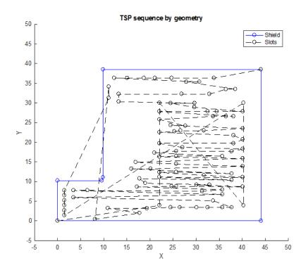
Fig. 8. Sequence by slots geometries, followed by the extruder to print layer 1.
