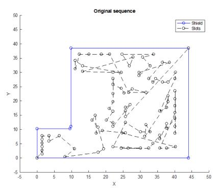
Fig. 7. Original Sequence followed by the printer to print layer 1.
