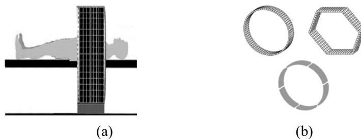
Fig. 1. PET scanner (a) model and (b) three different shapes of detector rings.
