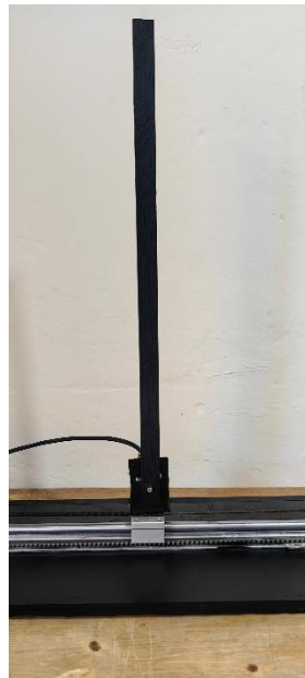
Fig. 2. Front view of the pendulum link and its coupling to the mobile carriage.
