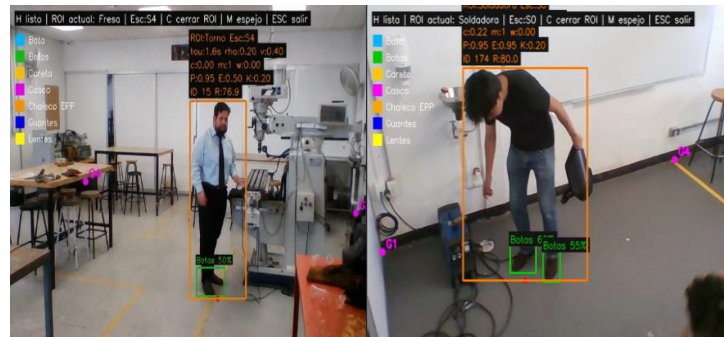
Fig. 11. Experimental evidence corresponding to Scenario S3 in the milling station (left), and Scenario S4 in welding station (right). The operators remain within the ROI for extended periods with some critical PPE equipment missing, resulting in increased exposure to hazardous areas and low PPE index.
