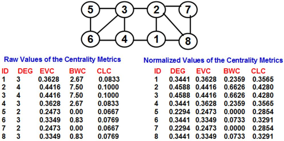
**Figure 2:** Example Graph as well as the Raw and Normalized Values for the Centrality Metrics
