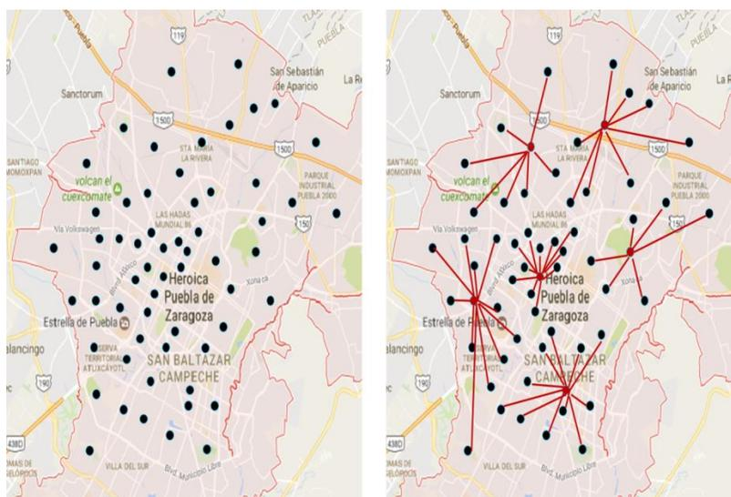
**Fig. 1.** Capacitated P-Median Problem (CPMP)
