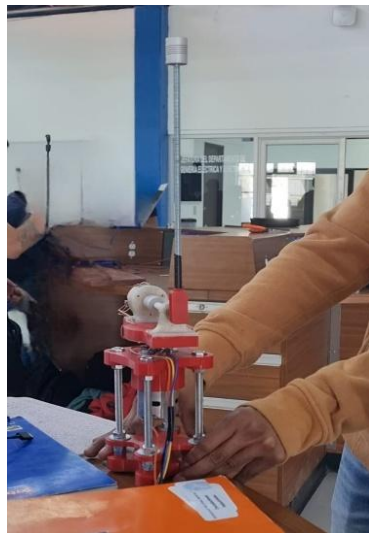
Fig. 3. Prototype of the Furuta pendulum designed and built for this work, in operation.
