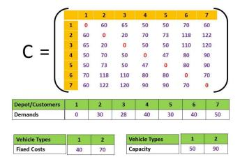
Figure 4: Sample problem's distance matrix, customer demands, vehicle types fixed costs and vehicle types capacity
