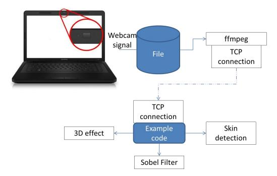
Fig. 7. Experimental arrangement for real time image processing, based on [7]
