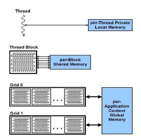
Fig. 2. Diagram of the nested levels of threads, blocks and grids, shows the corresponding levels of local, shared and global memory [25].
