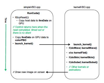
Fig. 9. Interaction between simpleVBO.cpp and the 3 Kernels [7]
