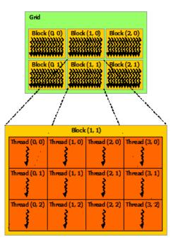
Fig. 1. Grid with a dimension of 2 x 3 blocks with a thread of 4 x 3 in the block [25].
