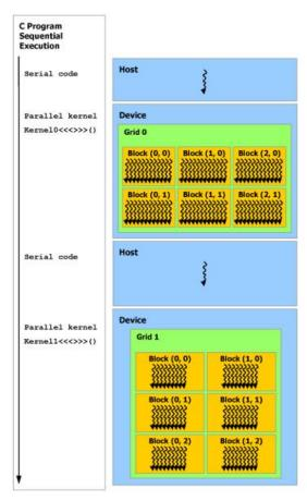
Fig. 4. Diagram showing that the sequential code is executed in the CPU and the parallelized code is executed in the GPU [25].
