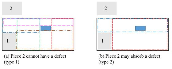
Figure 2: Residual Spaces when the next piece is from type 1 or type 2
