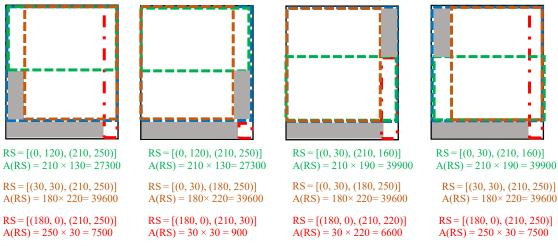
*Figure 6: Residual spaces generated when piece*  $p_2$  *is placed in*  $rs_1$  *with piece rotated (* $h_2 > w_2$ *).*
