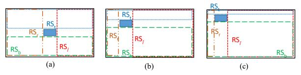
Figure 8: Different residual spaces created by a defect in a plywood sheet.
