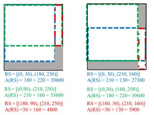
*Figure 7: Residual spaces generated when piece*  $p_2$  *is placed in*  $rs_2$  *with piece rotated (* $h_2 > w_2$ *).*
