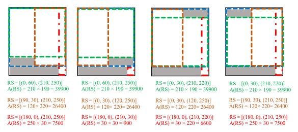
Figure 5: Residual spaces generated when piece  $p_2$  is placed in  $rs_1$  with original orientation ( $h_2 \le w_2$ ).
